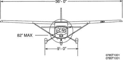
Figure 1-1. Three View - Normal Ground Attitude (Sheet 1 of 2)
