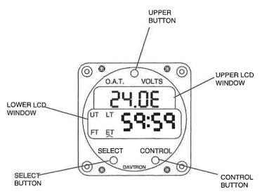
Figure 1. Davtron Model 803 Digital Clock
