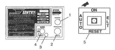
Figure 2. Pointer Model 4000-11 Emergency Locator Transmitter (ELT).
