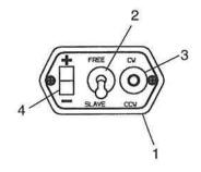
Figure 2. KA-51B Slaving Accessory and Compensator Unit
