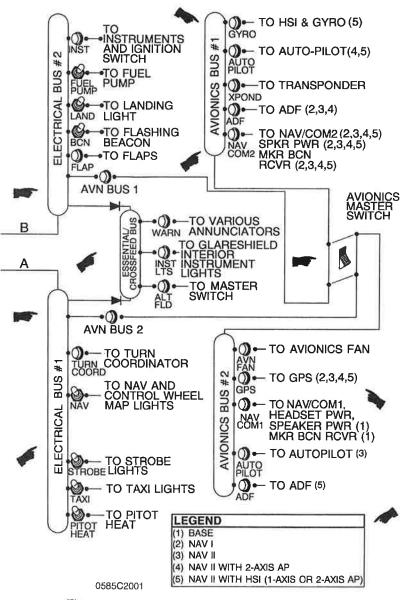
Figure 7-7. Electrical Schematic (Sheet 2 of 2)
