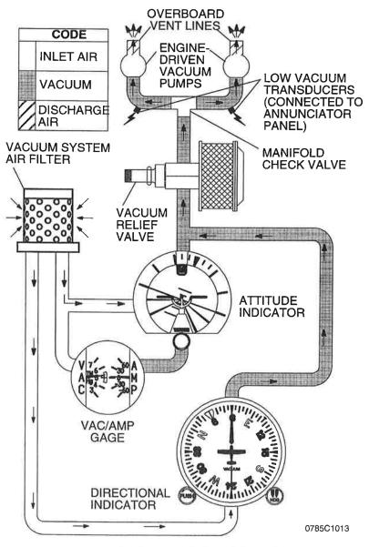
Figure 7-9. Vacuum System Schematic
