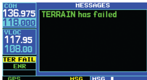
Figure 11-9: TERRAIN FAILED Display
