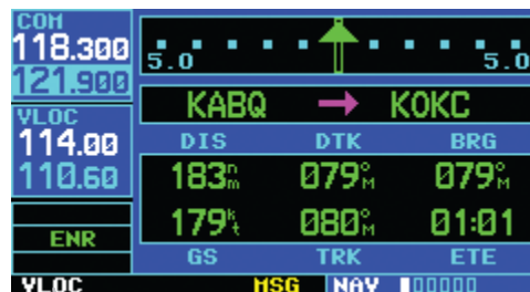
Figure 9-10 VLOC Coupled to External CDI
