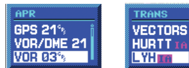
Figure 6-11 Approach and Transitions Windows
